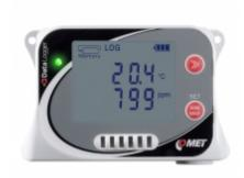
Datalogger is designed to record temperature, humidity, atmospheric pressure and CO2. In case of exceeded set limits alarms are indicated by LED, LCD and acoustically by built-in beeper.
