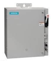
Pump control panel, Size 3, Three phase full voltage, Solid-state overload relay, OLR amp range 25-100A, 110V 50Hz / 120V 60Hz coil, Standard type contactor, 100A circuit breaker, HOA Sel Sw. <(>&<)> Start P.B., Enclosure NEMA type 3/3R, Weather proof outdoor use
