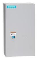
Reversing motor starter, Size 4, Three phase full voltage, Solid-state overload relay, OLR amp range 50-200A, 110V 50Hz / 120V 60Hz coil, Non-combination type, Enclosure type 1, Indoor general purpose use, Standard width enclosure
