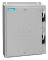
Duplex starter w/ alternator, Size 1, Three phase full voltage, Amb. compensate bimetal OLR, contactor A rating 27A, 110V 50Hz / 120V 60Hz coil, Combination type, Two 30A circuit breakers, Enclosure NEMA type 12, Dust/drip proof for indoors
