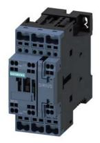
power contactor, AC-3 12 A, 5.5 kW / 400 V 1 NO + 1 NC, 125 V DC 3-pole, Size S0 Spring-type terminal
