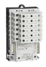
Electrically held lighting contactor, (convertible to mech. held), Amp rating 30A (tungsten 20A), 7 N.C. / 0 N.O. poles, 347V 60Hz coil, Non-combination type, Enclosure NEMA type (open), No enclosure
