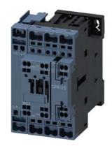
Contactor, AC-1, 40 A/400 V/40 °C, S0, 4-pole, 230 V AC, 50/60 Hz, 1 NO+1 NC, Spring-type terminal
