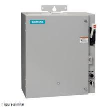
Pump control panel, Size 4, Three phase full voltage, Solid-state overload relay, OLR amp range 50-200A, 190-220/220-240V 50/60Hz coil, Standard type contactor, 200A fusible disconnect, 200A/250V fuse clip, HOA Sel Sw. <(>&<)> Start P.B., Enclosure NEMA type 3/3R, Weather proof outdoor use
