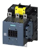
Power contactor, AC-3 150 A, 75 kW / 400 V Coil AC 50/60 Hz and DC 200-277 V x (0.8-1.1) F-PLC input 24 V DC 3-pole size S6 Auxiliary contacts 2 NO + 2 NC Main circuit: Busbar Control and auxiliary circuit: screw terminal
