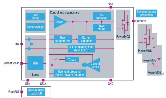
Note: (1) One to four integrated power MOSFETs, depending on the number of channels  $\,$
