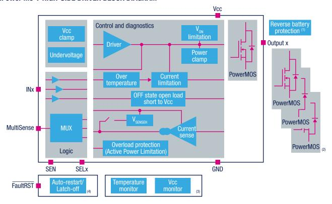
Note: (1) Built-in reverse battery protection, allowing self turn-on of the output power MOSFETs, available on selected devices
