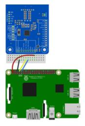
Pi 3V to breakout 3.3V Pi GND to breakout GND Pi RXD to breakout TX Pi TXD to breakout RX
