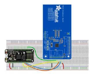
Board 3V to breakout 3.3V Board GND to breakout GND Board MISO to breakout MISO Board MOSI to breakout MOSI Board SCK to breakout SCK Board D5 to breakout SSEL
