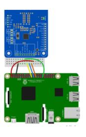
Pi 3V to breakout 3.3V Pi GND to breakout GND Pi MOSI to breakout MOSI Pi MISO to breakout MISO Pi SCLK to breakout SCK Pi D5 to breakout SSEL
