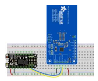
Board 3V to breakout 3.3V Board GND to breakout GND Board RX to breakout TX Board TX to breakout RX
