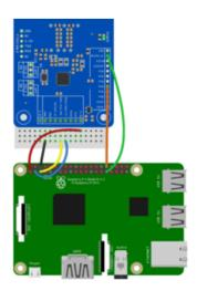
Pi 3V to breakout 3.3V Pi GND to breakout GND Pi SCL to breakout SCL Pi SDA to breakout SDA Pi D6 to breakout RSTPD\_N Pi D12 to breakout P32
