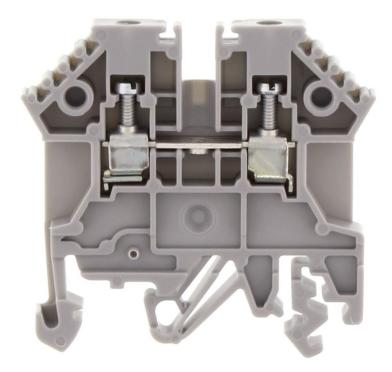
Feed-through terminal, Screw connection, Mounting type:Mounting rail TS 35/7.5 and TS 32, Rated cross-section: 2.5 mm<sup>2</sup>, Width: 5 mm, Colour: Grey
