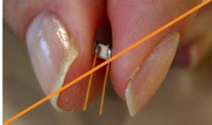
Picture 6: Sensor held with fingers without gloves on the active
