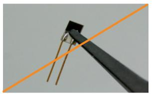
Picture 3: Sensor picked on the active area
