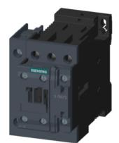
Contactor, AC-1, 40 A/400 V/40  $^\circ\text{C},$  S0, 4-pole, 125 V DC, 1 NO+1 NC, screw terminal
