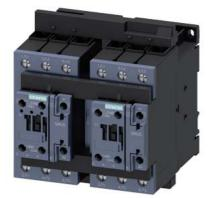
Reversing contactor assembly for 3RA27 AC-3, 22 kW/400 V, 20-33 V AC/DC 3-pole, Size S2 screw terminal electrical and mechanical Interlock 2 NO integrated with voltage tap
