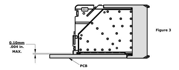
There should be no broken standoffs along the perimeter of the part (an indication of overpressing).
