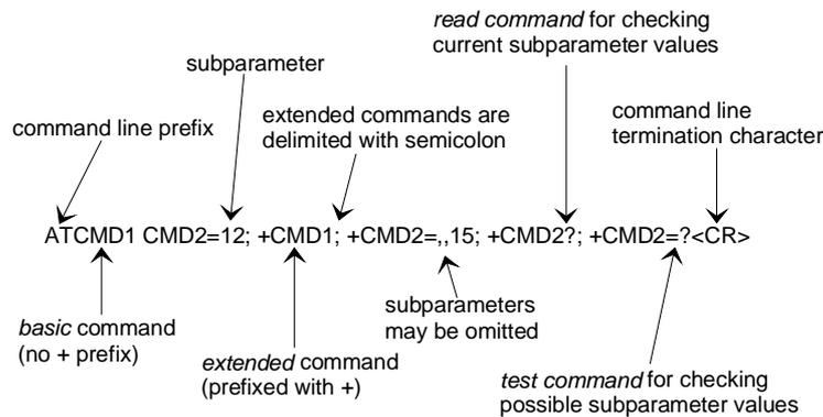
Figure 2: Basic structure of a command line
