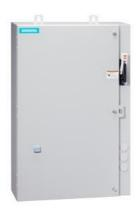
Reversing motor starter, Size 3, Three phase full voltage, Solid-state overload relay, OLR amp range 25-100A, Combination type, 125A circuit breaker, Enclosure NEMA type 4/12, Water/dust tight for outdoors
