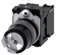
RONIS key-operated switch, 22 mm, round, plastic with metal front ring, lock number SB30, with 2 keys, 2 switch positions O-I, latching, actuating angle 90°, 10:30h/13:30h, key removal O+I, with holder, 1 NO, screw terminal, possible special locks: SB31, 421, 455, with laser labeling, inscription or symbol Customer-specific selection with SIRIUS ACT configurator (CIN)
