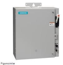
Pump control panel, Size 3, Three phase full voltage, Solid-state overload relay, OLR amp range 25-100A, 190-220/220-240V 50/60Hz coil, Standard type contactor, 100A fusible disconnect, 100A/250V fuse clip, HOA Sel Sw. <(>&<)> Start P.B., Enclosure NEMA type 3/3R, Weather proof outdoor use
