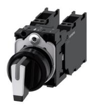
Selector switch, illuminable, 22 mm, round, plastic, white, selector switch, short, 3 switch positions I>O<II, momentary contact type, 10:30h/12h/13:30h, with holder, 2 x 1 NO+1 NC, spring-type terminal, with laser labeling, upper case
