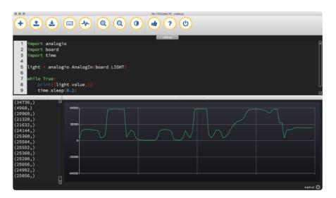
Note you can have the text REPL on the left and resize the plotter to be big and on the right like above. That way you see the numbers and the graph at the same time. The plotter will automatically re-scale depending on light levels.
