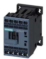
power contactor, AC-3 12 A, 5.5 kW / 400 V 1 NC, 24 V AC, 50 / 60 Hz 3-pole, Size S00 Spring-type terminal upright mounting position
