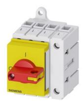
Load disconnector 3LD3, lu 32 A Main switch 3-pole + N Rated operating capacity for AC-23 A at 400V 11.5kW Installation in distribution boards, Basic switch with selector knob red / yellow
