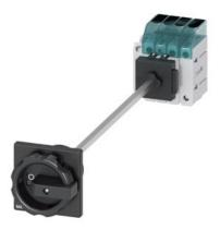
Load disconnector 3LD3, lu 25 A Main switch 3-pole + N Rated operating capacity at AC-23 A at 400V 9.0kW floor mounting Basic switch with door coupling Central hole mounting 22.5mm Rotating drive black 66 x 66 mm with auxiliary switch 1OE + 1S
