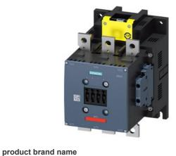
Power contactor, AC-3 300 A, 160 kW / 400 V Coil AC 50/60 Hz and DC 96-127 V x (0.8-1.1) F-SPS input 24 V DC 3-pole size S10 Auxiliary contacts 2 NO + 2 NC permanently mounted Main circuit: Busbar Control and auxiliary circuit: Screw terminal
