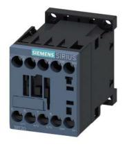
Power contactor, AC-3 7 A, 3 kW / 400 V 1 NC, 24 V DC 3-pole, Size S00 screw terminal upright mounting position
