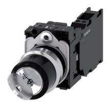
RONIS key-operated switch, 22 mm, round, metal, shiny, lock number SB30, with 2 keys, 2 switch positions O-I, latching, actuating angle 90°, 10:30h/13:30h, key removal O+I, with holder, 1 NO+1 NC, spring-type terminal, possible special locks: SB31, 421, 455 upper case and lower case, always upper case at the beginning of the word
