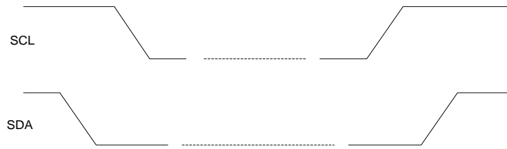
Figure 34: I 2 C START and STOP Conditions
