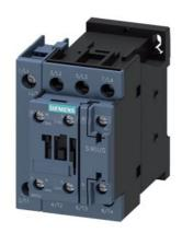
Contactor, AC-1, 40 A/400 V/40 °C, S0, 4-pole, 24 V AC/50 Hz, 1 NO+1 NC, screw terminal
