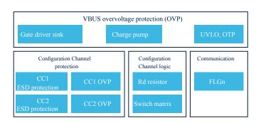
Figure 3. Internal block diagram
