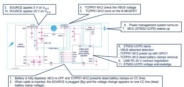
Figure 17. Wake-up sequence in dead battery condition
