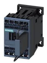
traction contactor, AC-3 12 A, 5.5 kW / 400 V 24 V DC, 0.7-1.25\*US with integrated suppressor diode 3-pole, size S00 spring-type terminal suitable for PLC outputs not expandable with auxiliary switch
