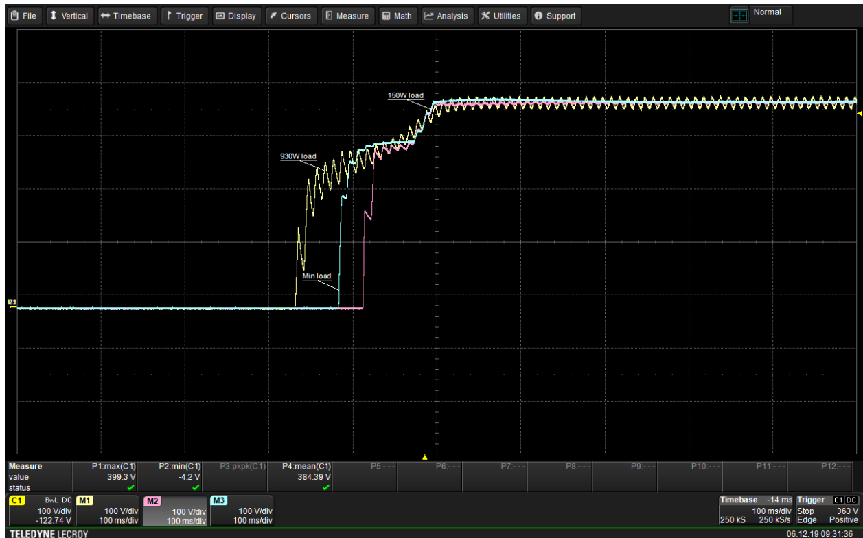
Figure 12. Start up to Open Circuit, 155 W and 930 W at 230 V AC Input
