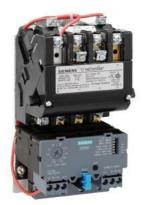
Non-reversing motor starter Size 00 Three phase full voltage Solid-state overload relay OLRelay amp range 3-12A 24VAC 50-60HZ coil Combination type No enclosure
