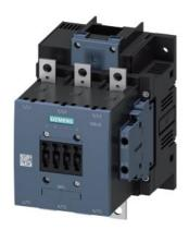
Contactor, AC-1, 275 A/690 V/40  $^{\circ}$ C, S6, 3-pole, 42-48 V AC/DC, with varistor, 2 NO+2 NC, Connection rail/ screw terminal
