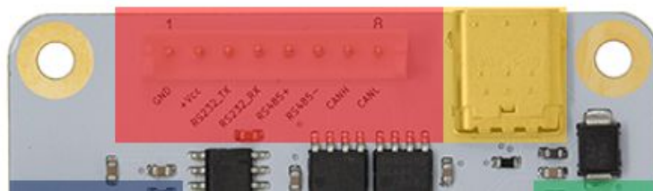
Figure 3: Power / communication connector of TMCM-0960-MotionPy V21
