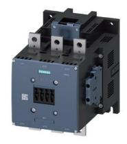
Contactor, AC-1, 690 A/690 V/40 °C, S12, 3-pole, 21-27.3 V AC/DC, PLC-IN optional, with varistor, 2 NO+2 NC, Connection rail/ screw terminal
