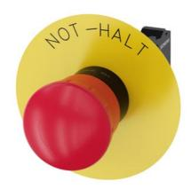
EMERGENCY STOP mushroom-type actuator, 22 mm, round, plastic, red, 40 mm, positive latching, according to EN ISO 13850, rotate-to-unlatch, with yellow backing plate, inscription: NOT-HALT, with holder, 1 NC, spring-type terminal, Z=20-unit packaging
