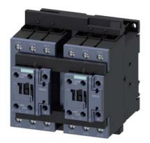
Reversing contactor assembly AC-3,18,5kW/400V,AC110V,50/60Hz 3-pole, Size S2 screw terminal electrical and mechanical Interlock 2 NO integrated
