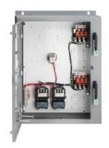
Pump control panel, Duplex controller NEMA size 1 Solid-state overload relay, OLR amp range 3-12A, 120 VAC coil, Fusible disconnect HOA Sel Sw. and Start P.B., Enclosure NEMA type 3/3R,12 Weather proof outdoor use
