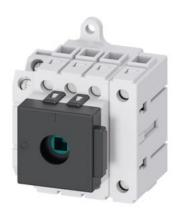
Load disconnector 3LD3, lu 40 A Main switch 3-pole + N Rated operating capacity at AC-23 A at 400 V 18.5 kW Installation in distribution boards, Basic switch without Knob-operated mechanism with auxiliary switch 1OE + 1S
