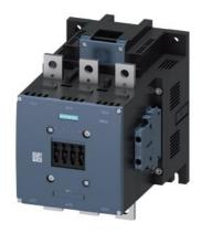
power contactor, AC-3 400 A, 200 kW / 400 V AC (50-60 Hz) / DC operation 380-420 V AC/DC auxiliary contacts 2 NO + 2 NC 3-pole, frame size S12 busbar connections drive: conventional screw terminal
