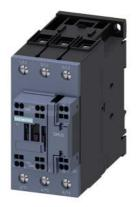
Power contactor, AC-3 65 A, 30 kW / 400 V 1 NO + 1 NC, 230 V AC 50/60 Hz, 3-pole Size S2, Spring-type terminals
