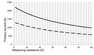
$\label{eq:UC} \begin{array}{l} ---- U_C = \pm 24 \; V \; -5 \; \%, \; T_A = 85 \; ^\circ C \\ ---- U_C = \pm 15 \; V \; -5 \; \%, \; T_A = 85 \; ^\circ C \\ \\ \mbox{Primary currents higher than } I_{PM} \; \mbox{only for peak!} \end{array}$
