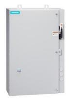
Non-reversing motor starter, Size 1 3/4, Three phase full voltage, Solid-state overload relay, OLR amp range 10-40A, Combination type, 60A fusible disconnect, 60A/250V fuse clip, Encl NEMA type 4X 304 S-Steel, Water/dust tight noncorrosive, Extra-wide enclosure
