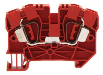
Feed-through terminal, Tension-spring connection, Mounting type: Mounting rail TS 35/7.5, Rated cross-section: 6 mm<sup>2</sup>, Width: 8.1 mm, Colour: Red
