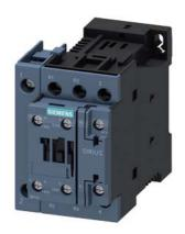
Power contactor, AC-3 25 A, 11 kW / 400 V 2 NO + 2 NC 12 V DC 4-pole size S0 screw terminals 1 NO + 1 NC integrated
