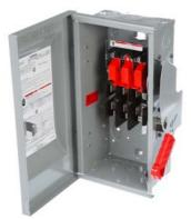
Siemens Low Voltage Circuit Protection Heavy Duty Safety Switches. Type: ENCLOSED, SAFETY SWITCH Std: UL V. Rating: 240V A. Rating: 30 A Wattage: 4W No. Of Poles: 3P F. Rating: 60Hz Action: SINGLE THROW Material: STEEL Enclosure: TYPE 1. 2-3 point mounting holes. O. Cycles: 10000 O. Temperature: (-20F-120F) AMBIENT TEMPERATURE Environmental Conditions: INDOOR
