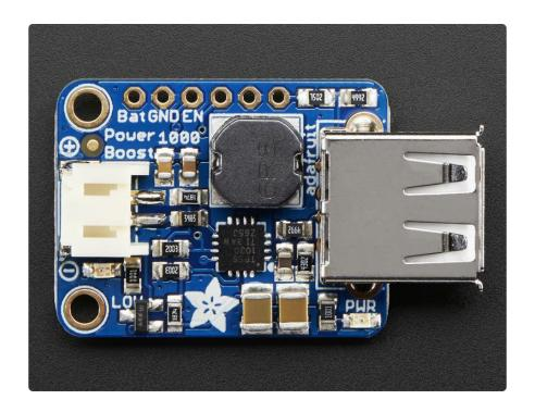
The PowerBoost 1000 has at the heart a <u>TPS61030 boost converter from TI</u> (). This boost converter chip has some really nice extras such as low battery detection, 4A internal switch, synchronous conversion, excellent efficiency, and 700KHz high-frequency operation. Check out these specs!
