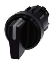
Illuminable selector switch, 22 mm, round, plastic, black, Selector switch short, 3 switch positions I-O-II, latching, actuating angle 2x45°,  $10:\!30h/12h/13:\!30h$
